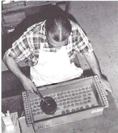
Arthur Cesati potting a tray of 1592 type inductors. The potting gun is filled with liquid wax. Each inductor shell is sealed by filling it with wax.
