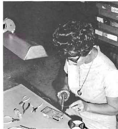
June Caron shown assembling a 1592 type inductor into a 475A network. The networks, still in department 973 are washed and tested before being released.
