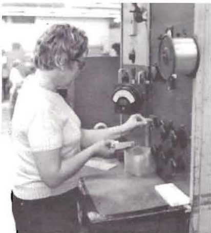
Victoria Flynn testing the completed inductors after they have passed visual inspection. Each inductor must supply exactly the required inductance value.
